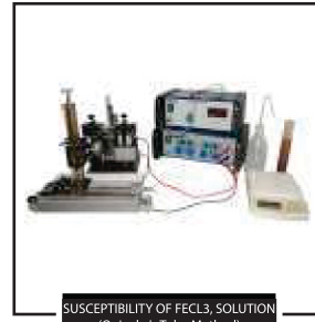
SUSCEPTIBILITY OF FeCl_3 SOLUTION (Quinke's Tube Method)
